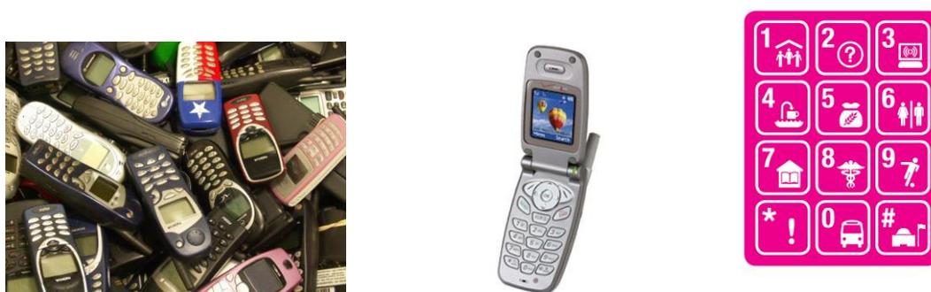
Fig. 2. The virtual “town center” hardware: fitting out a recycled feature cell-phone to include a new keypad showing universal icons and numbers designating essential services such as water, information, food, medical assistance, Internet access, etc. The cell-phone in the hands of individuals send information and essential feedback from the inside to coordinated expertise seeking to help.
